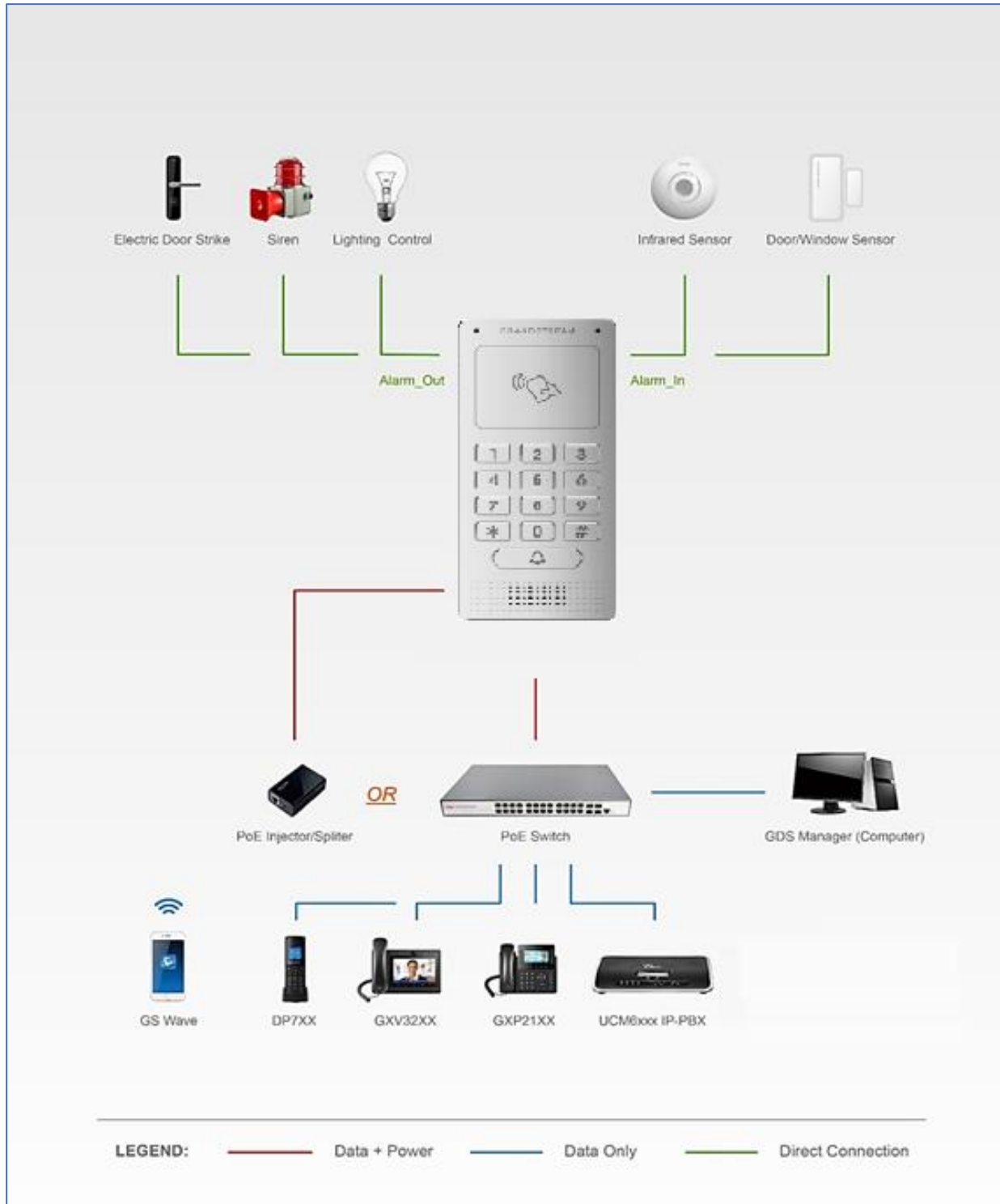
Figure 14: Peripheral Connections for GDS3705
