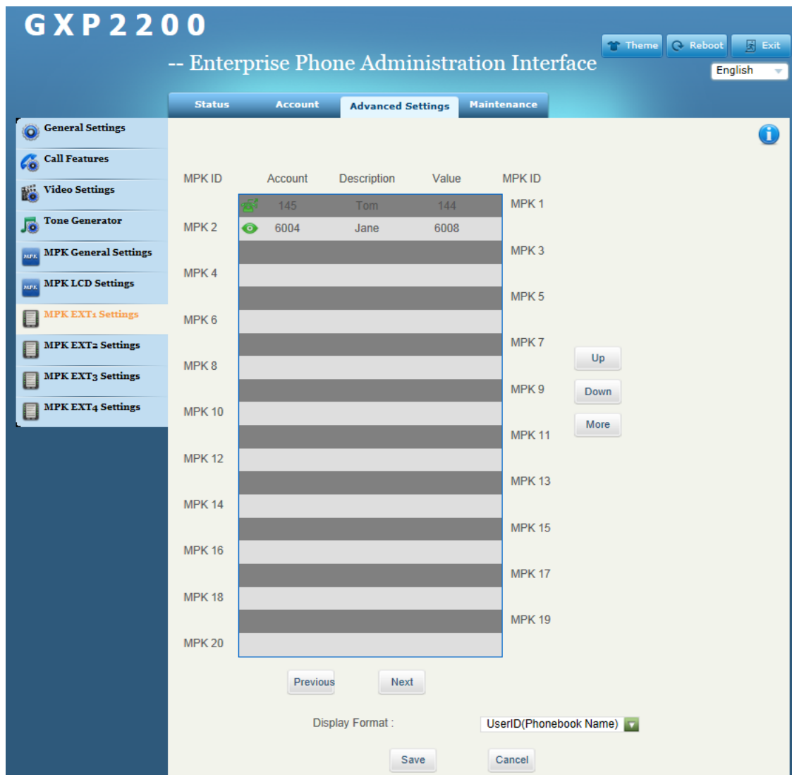
Figure 9: GXP2200 Extension Board Configuration via GXP2200 Web GUI
